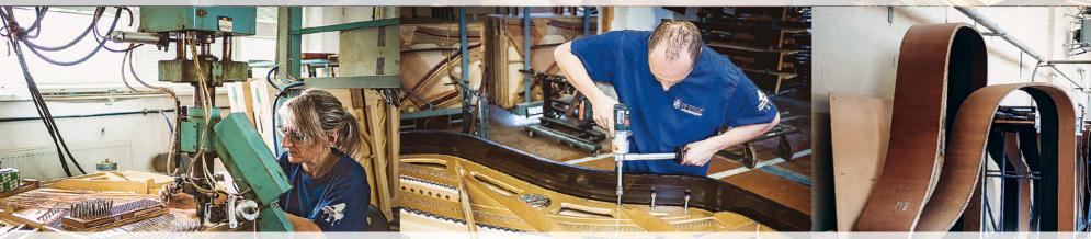
onto the piano frame is partly carried out using a machine that ensures the correct height of the tuning pins and the required number of turns for the strings. strings, which this construction has to bear, can in a grand piano reach over 20 tonnes. construction.
